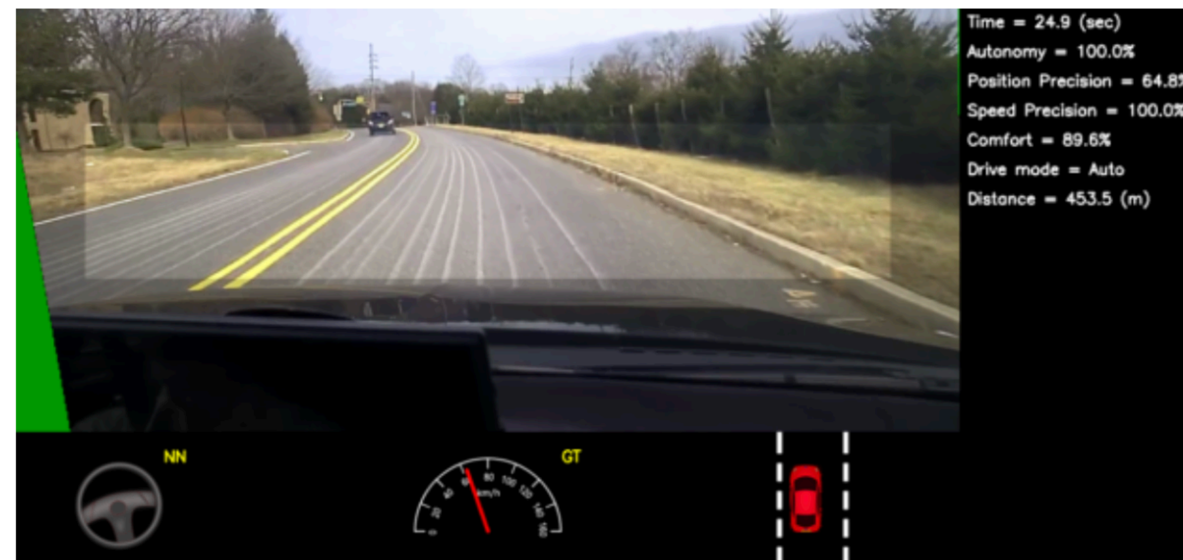
Figure 7: Screenshot of the simulator in interactive mode. See text for explanation of the performance metrics. The green area on the left is unknown because of the viewpoint transformation. The highlighted wide rectangle below the horizon is the area which is sent to the CNN.
